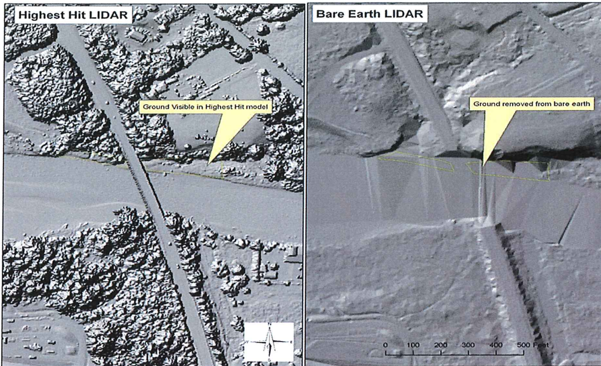
Figure 6: Example of missing ground in lidar DEM hillshaded raster. Ground is clearly visible in highest hit model, but has been removed from the bare earth model. This type of classification error is common near water body features
